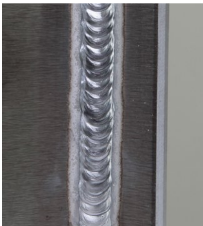
AlMg5, material thickness: 4 mm
