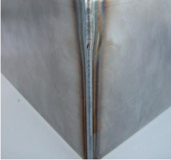
Welding unalloyed sheet metal
